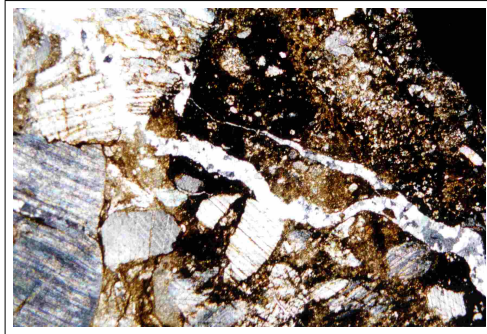
TS JEN-7 N36372 XN x13. Breccia of limestone, goethite and ferruginised, altered ?dolomite.
