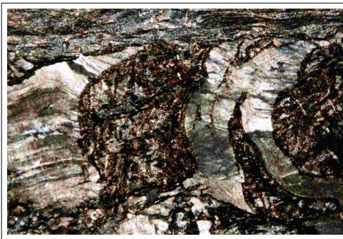
TS J58/24 N35755 XN x13. Fault-zone breccia with spar and suspected chert fragments.
