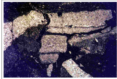
TS J105/4 XN 3.2x. Large bioclasts suspended in a matrix of dedolomite and opaques.
