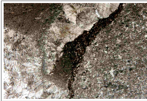
TS JEN-10A N36451a PPL x13. Acicular (calcite) cement (LHS) may have been originally aragonite or gypsum.
