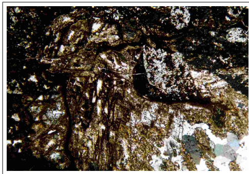
TS J58/5 XN x3.2. Breccia of dolomite, possible dyke fragments and pyrolusite.
