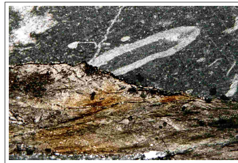
TS J58/24 N35755 PPL x13. Fault zone breccia with stretched argillite and limestone
